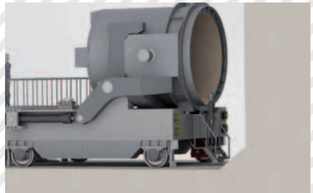
8. Ladle transfer car Ladle transfer car
