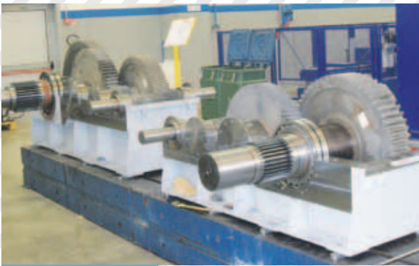
9. Collaudo riduttori Gearbox Testing
